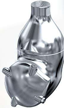
The Bio 10 rotary jet head is a hygienic tank cleaning machine that provides 360deg coverage within a given tank or process vessel. It is self powered by the flow of the fluid through the inlet cone of the machine. An increase in pressure and flow will correspondingly increase the length of the jet and impact upon the tank or vessel surfaces.
