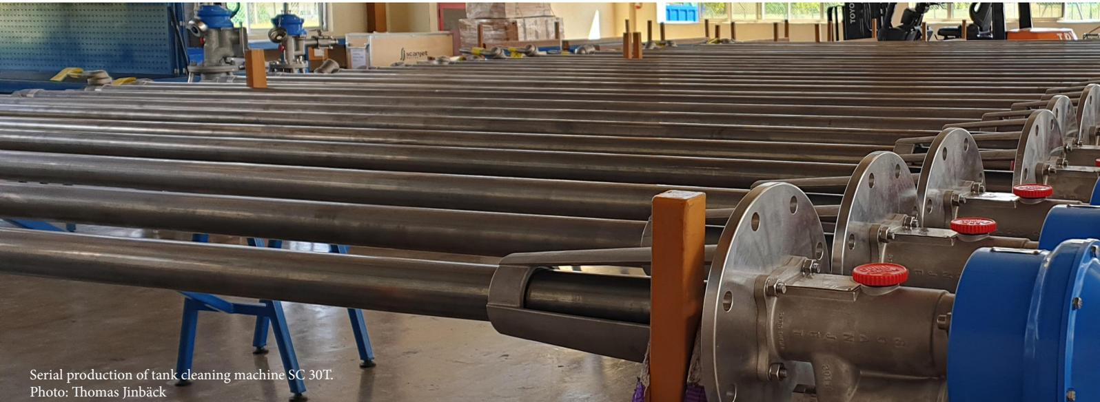
Serial production of tank cleaning machine SC 30T.
