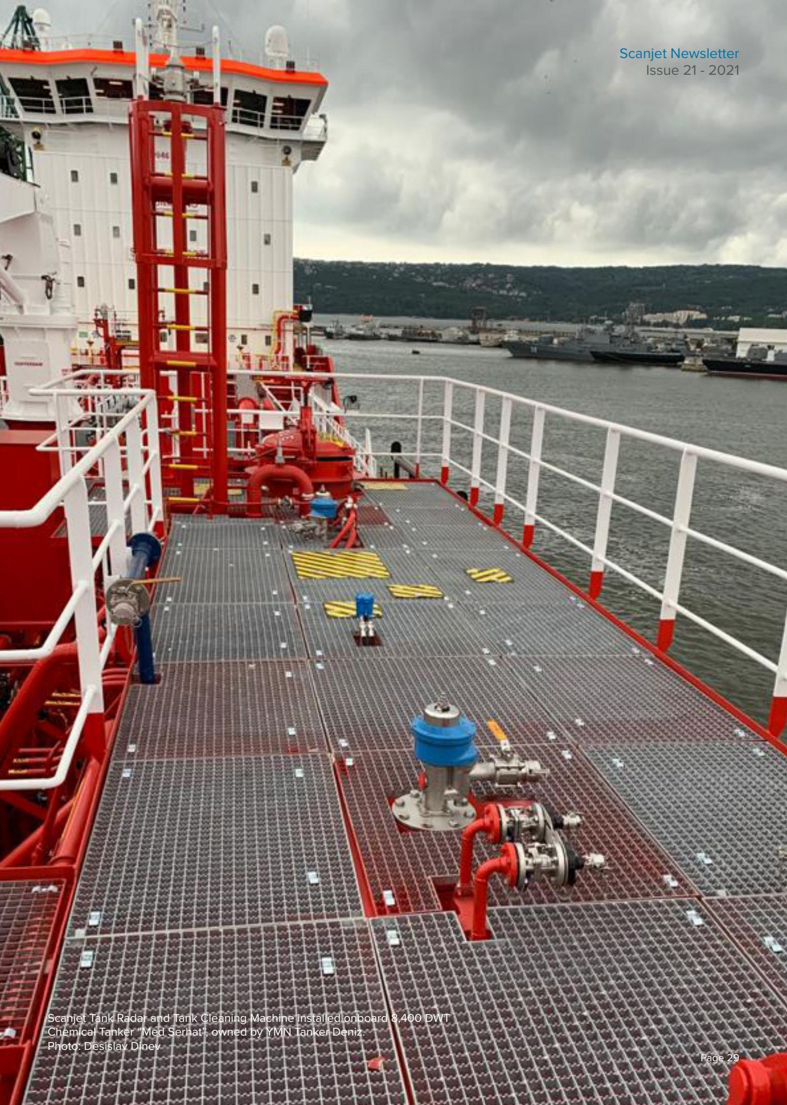
Scanjet Tank Radar and Tank Cleaning Machine installed onboard 8,400 DWT Chemical Tanker "Med Serhat", owned by YMN Tanker Deniz.
